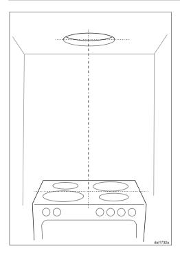
■ Cut a 7 <sup>1</sup>/<sub>2</sub>" (190 mm) hole in the ceiling centered over the cooktop for the exhaust duct to pass through.
